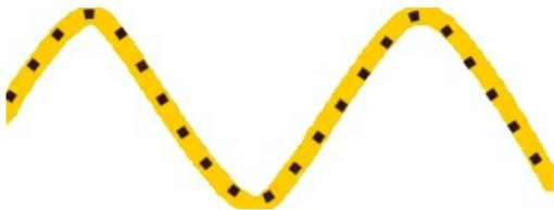
Each dot in the figure above represents one audio *sample*. The more samples per second, the more accurate the mapping of the electrical wave.
